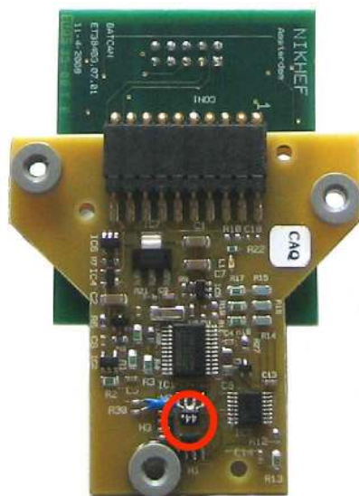
Figure 5. One of the cards with its readout electronics is shown. The red circle in the picture indicates the three orthogonal Hall probes which are placed on a small glass cube.
