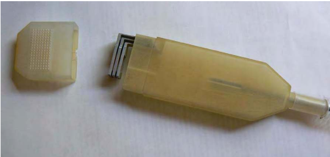
Figure 70: Telescope mechanical housing and positioning head. The MIMOSTAR-2 flex cables will be glued to the aluminum support and positioning brackets.
