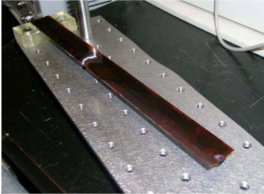
Figure 51: Early prototype ladder and detector carrier.
