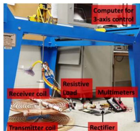
Figure 6. Experimental setup for misalignment study.
