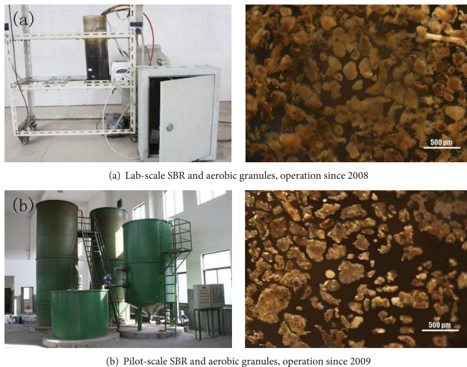
FIGURE 2: Photographs of reactors and sludge of lab-scale SBR and pilot-scale SBR in Yancang WWTP.
