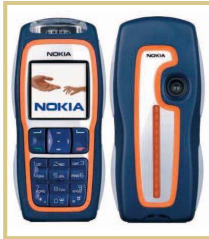
Figure 6. The Nokia 3200 cell phone features a Near Field Communications reader. From the front, it looks like an ordinary cell phone, but on the back, you can see the reader coil molded into the housing. (figure courtesy of Nokia)
