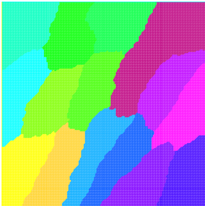
FIGURE 6. Subdomain partitioning into 16 subdomains using METIS.
