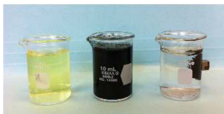
FIGURE 3: Adsorption experiment. From left to right: dissolution of tartrazine, mixture of tartrazine with magnetic modified carbon, and magnetic support separation.
