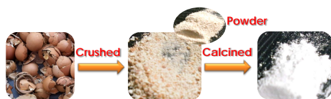
Figure 1. Preparation of CaO catalyst derived from eggshell waste
