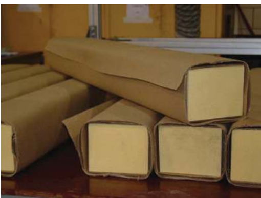
Figure 14: Paper wrapped on foam core ready to be assembled in the preform [32].
