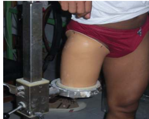
Figure 12: Static comfort test of socket prosthesis [25].
