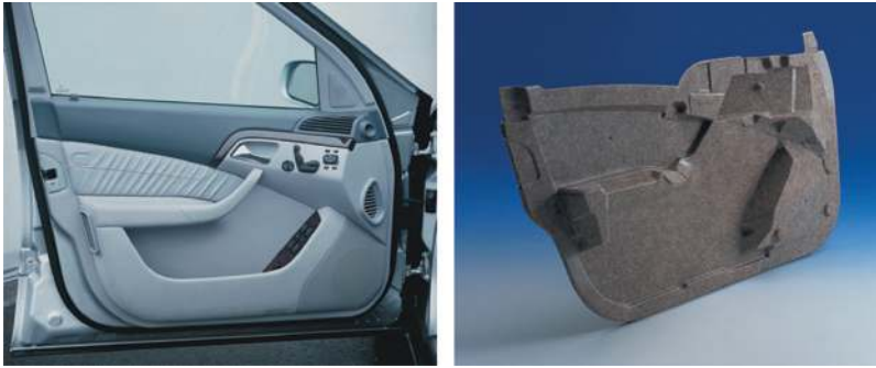
Figure 4: These modern door inner trim panels are molded using mats of 60% natural fiber in a Baypreg polyurethane resin (Courtesy of Bayer Polymers) [15].
