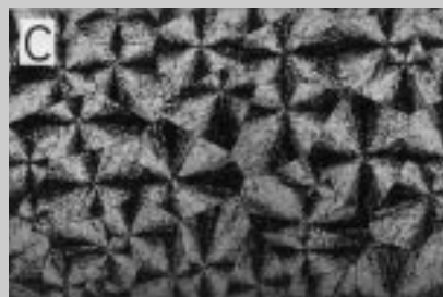
Polarizing optical photomicrograph of a PLLA film annealed at 140 °C after melting at 200 °C
