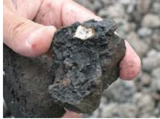
FIGURE 4: Gravel-size steel slag particle with a lime pocket (photograph taken at Mittal Steel, Indiana Harbor West Plant).
