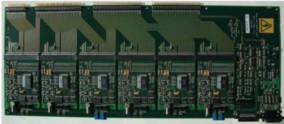
Figure 18. The VFE AHCAL base board with six mezzanine boards. The connection to the SiPMs is via coaxial cables.
