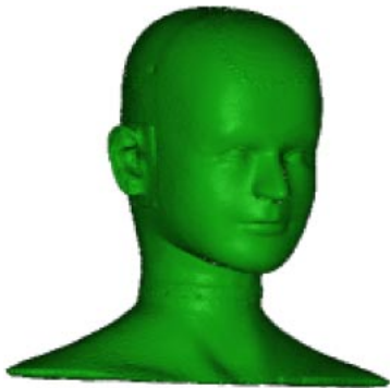
Fig. 2 Example of three-dimensional shading applied to the mesh data. The original data were measured using a three-dimensional scanner (VIVID910, Konica Minolta) and were saved in stereolithography (STL) format consisting of numerous meshes composed of triangulated surfaces.
