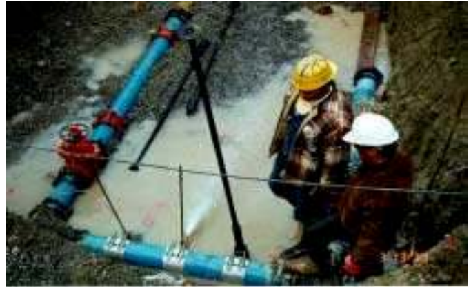
Leak detection tests used an experimental water pipe at a facility constructed especially for this project. Use of this site eliminated the public health risk and inconvenience normally associated with such tests.
