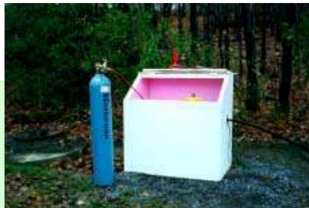
In the tracer gas method, a portable gas sensor is used to detect nontoxic gas as it escaped through leaks in the pipe and rises through the surrounding soil to the ground surface
