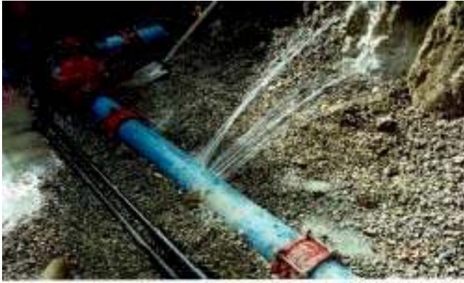
Leak detection tests used an experimental water pipe at a facility constructed especially for this project. Use of this site eliminated the public health risk and inconvenience normally associated with such tests.
