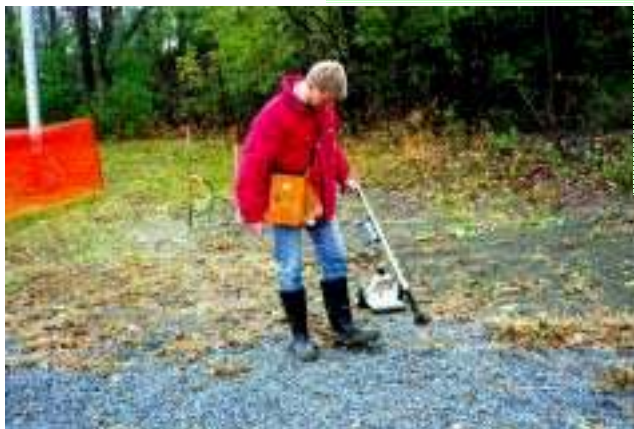
In the tracer gas method, a portable gas sensor is used to detect nontoxic gas as it escaped through leaks in the pipe and rises through the surrounding soil to the ground surface
