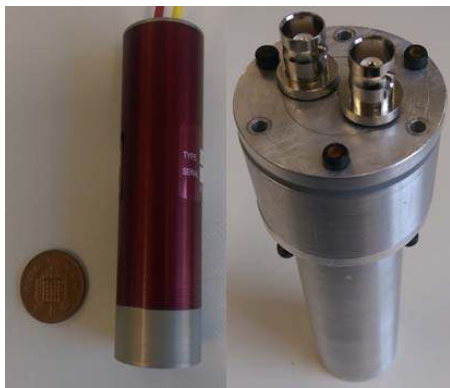
Fig. 4. Photograph of the CeBr 3 inorganic scintillation detector, without aluminum casing (left) and with aluminum casing (right), with a U.K. new penny of diameter 20 mm included far left for scale [8].
