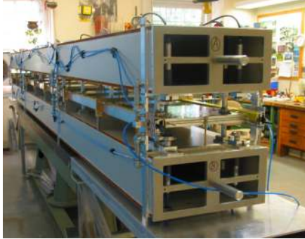
Figure 2. Glueing of a detector module box using the tool described in the text. The straightness of a 5 m long box built with that tool is shown. The rms of the deviation from a straight line is better than 400 \mu\text{m} .
