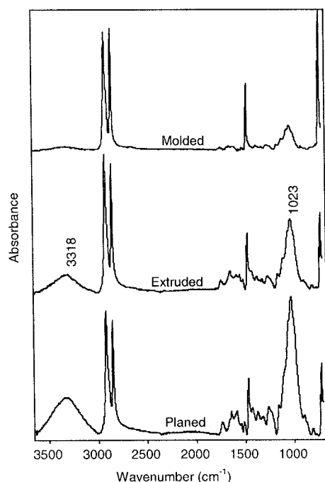
Figure 3 FTIR spectra of injection-molded, extruded, and planed WF/HDPE composites.
