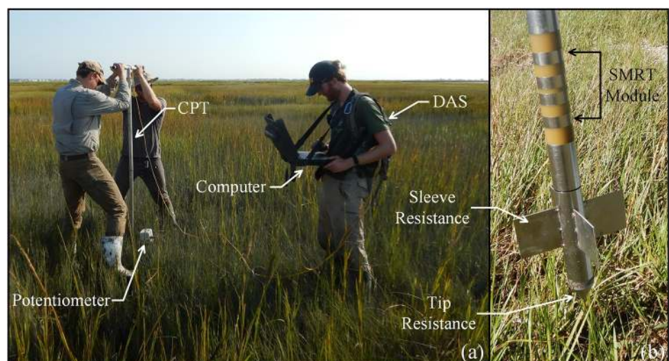
Fig 2. (a) Performing a cone penetrometer test and (b) cone penetrometer components.
