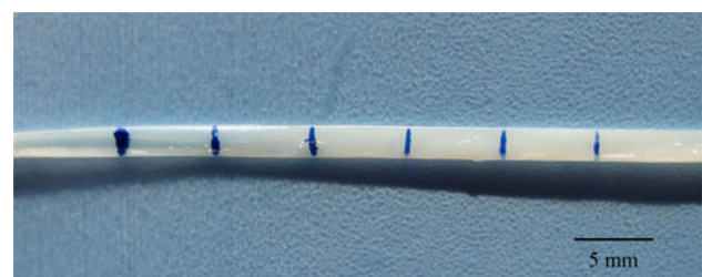
Fig. 2 Artery stretched at its physiological longitudinal stretch \lambda_z marked every 6 mm using dark ink
