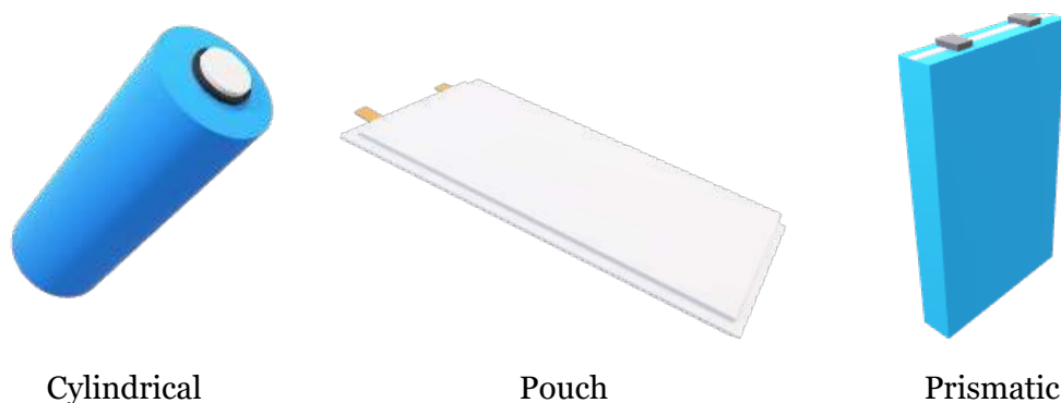
Figure 11 Exterior housing types that are common for lithium-ion battery cells.
