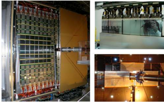
Figure 1: View of the TT installed in LHCb (left). View of the first IT station (bottom right), and detail of one of the detector boxes (top right).
