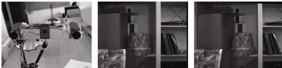
Figure 3 The Time-Of-Flight stereo rig and the rectified image pair I_l and I_r used in the experiment
