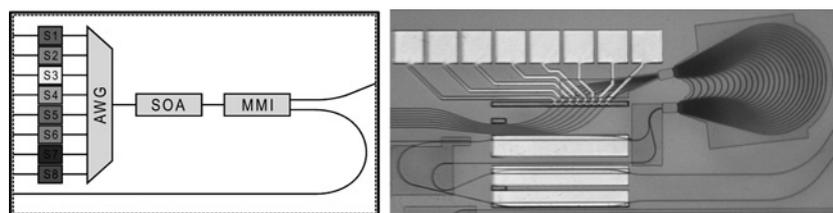
Fig. 2 Circuit scheme and microscope photograph of an AWG-based fast tunable laser, which has been realised in the COBRA InP-based generic integration process
