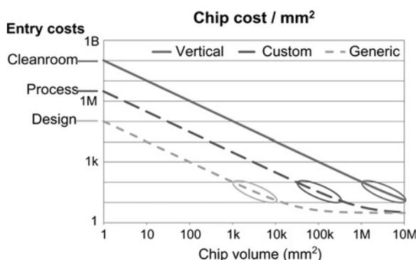
**Fig. 4** Illustration of the dependence of chip cost (per  $\text{mm}^2$ ) on the total chip volume (in  $\text{mm}^2$ ) for three different manufacturing models
