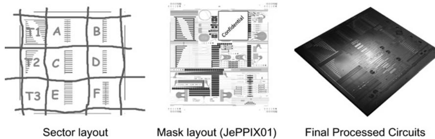
**Fig. 3** Example of a MPW realised in the COBRA process
