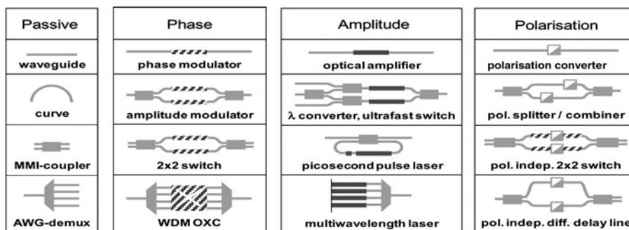
Fig. 1 Example of the functionalities that can be realised in a generic integration technology that supports four basic building blocks: passive waveguide devices, (optical) phase modulators, semiconductor optical amplifiers and polarisation converters
