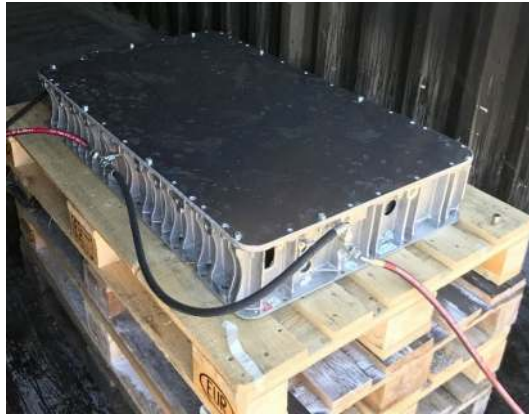
Figure 9. The second battery pack layer was removed for the remaining tests. Here the hoses connecting to nozzles inside the battery pack are also shown.
