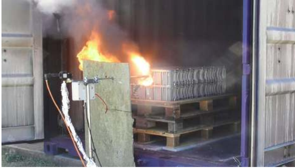
Figure 13. Thermal runaway event during test 1 (ref 1). This occurred after the flame impinged on the initiating module for roughly 20 min.
