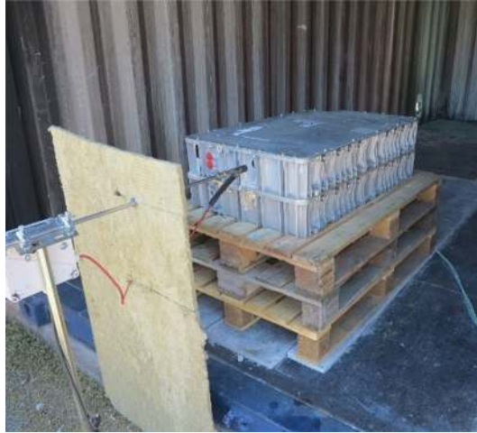
Figure 8. The battery pack consisting of two layers placed inside the test container. The burner used to initiate thermal runaway is also shown.
