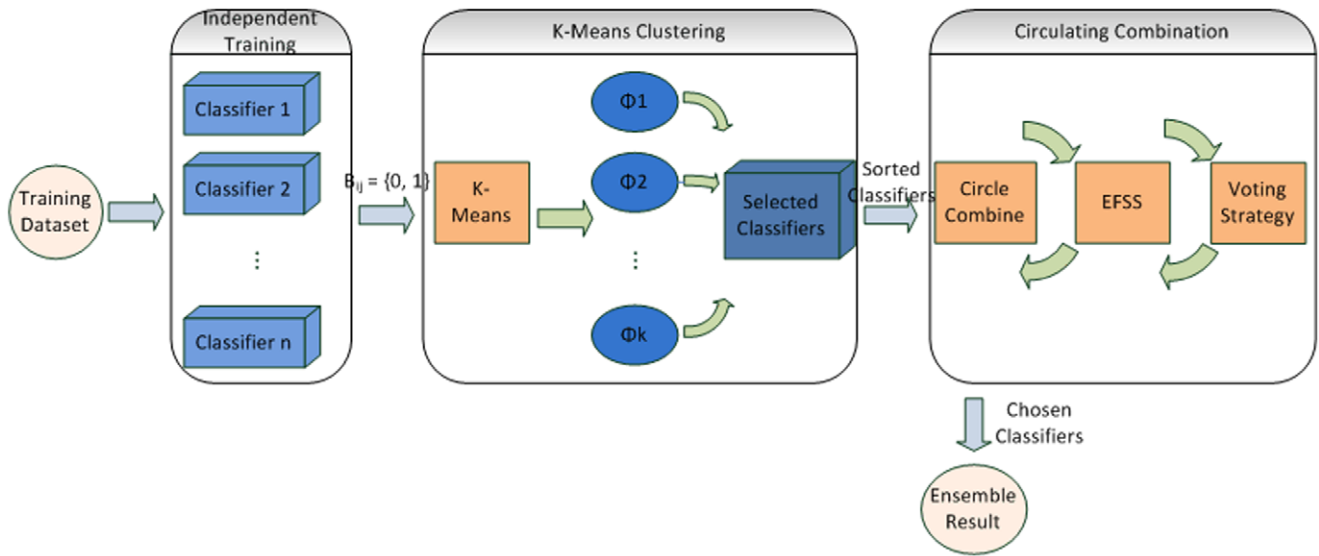
Figure 2. The architecture of our ensemble classifier. The training dataset is classified by all base classifiers. After K-Means clustering and circulating combination the best ensemble result is achieved. doi:10.1371/journal.pone.0056499.g002
