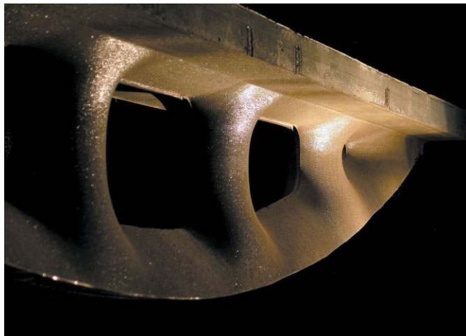
Fig. 21. Fabric-formed truss fabricated at C.-A.-S.-T.
