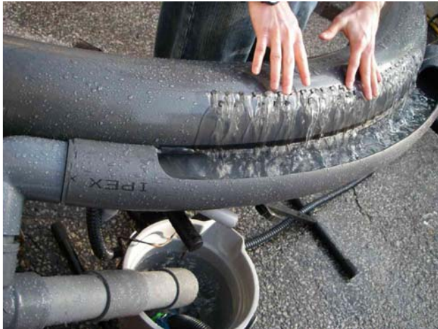
Figure 6: Portable lightweight 45-jet hydraulophone made from IPEX PVC pipe, with catch trough to recirculate the water into a bucket.
