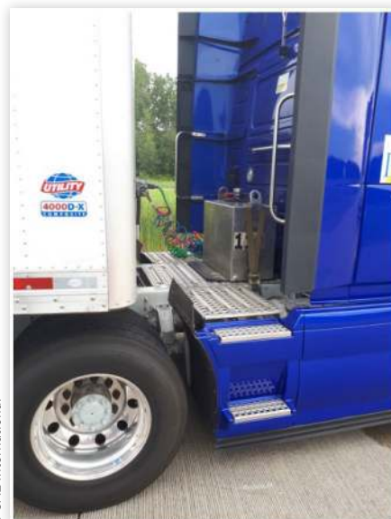
FIGURE 9 Installation of the portable fuel tanks.
