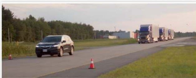
FIGURE 7 Mid-size SUV for “other traffic” and “cut-in” testing, shown leading 3-truck string with a 58 m separation distance to the lead truck (separation distance of 12 m between trucks).
