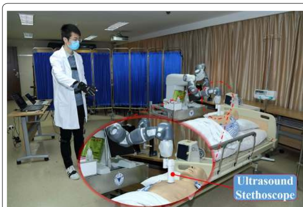
Figure 3 Remote auscultation using a Doppler Ultrasound Stethoscope based on the teleoperated robot
