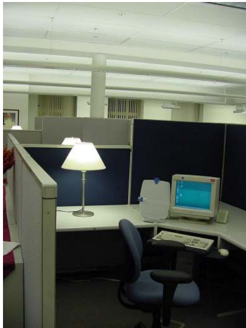
Figure 13. The desk lamp used in Lighting Design 3 (Best Practice with Switching Control).
