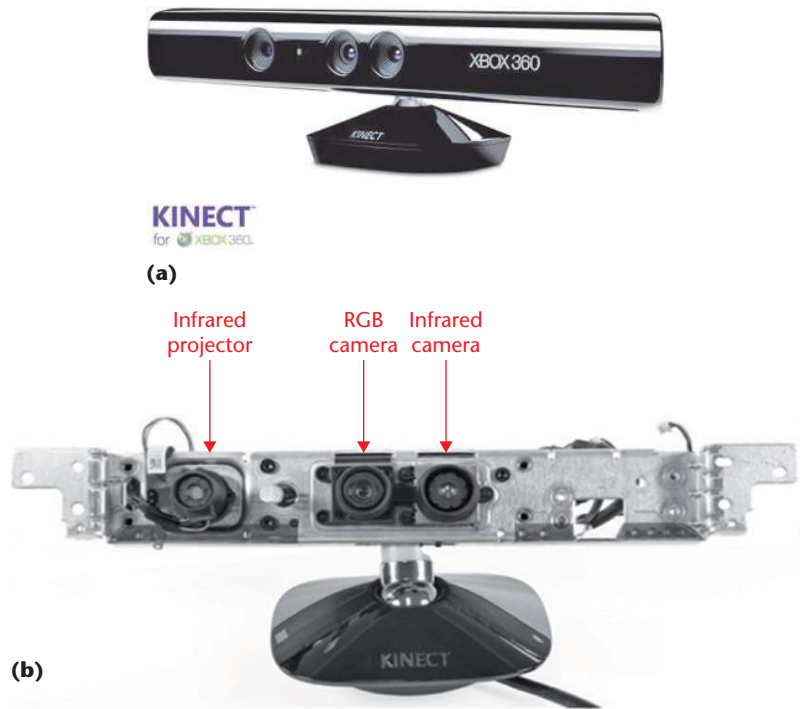
Figure 1. Microsoft Kinect sensor. (a) The Kinect sensor for Xbox 360. (b) The infrared (IR) projector, IR camera, and RGB camera inside a Kinect sensor.
