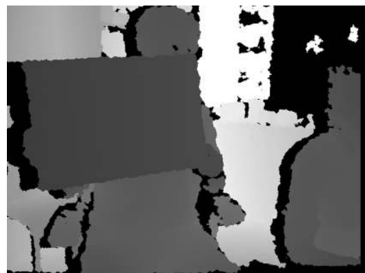
Figure 3. Kinect sensor depth image. The sensor produced this depth image from the infrared (IR) dot image in Figure 2.
