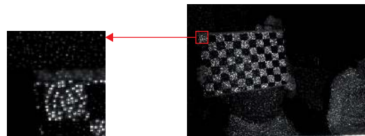
Figure 2. The infrared (IR) dots seen by the IR camera. The image on the left shows a close-up of the red boxed area.
