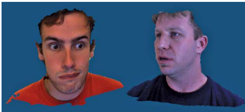
Figure 11. A screen shot of two remote people viewed from a third location. An enhanced 3D capture device runs in real time with multiple infrared (IR) projectors, IR cameras, and RGB cameras.
