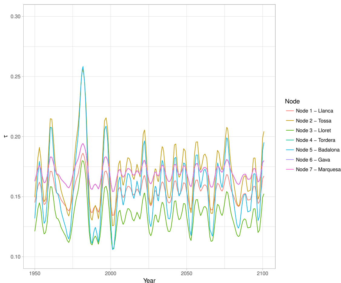
Figure 14. Strategy #2. Dependence parameter \tau of the Gumbel Archimedean copula at different model points, under the climate change scenario RCP8.5. Each color line represents a node from Figure 1.
