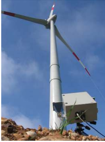
FIGURE 7: Radar measurement of a wind tower.
