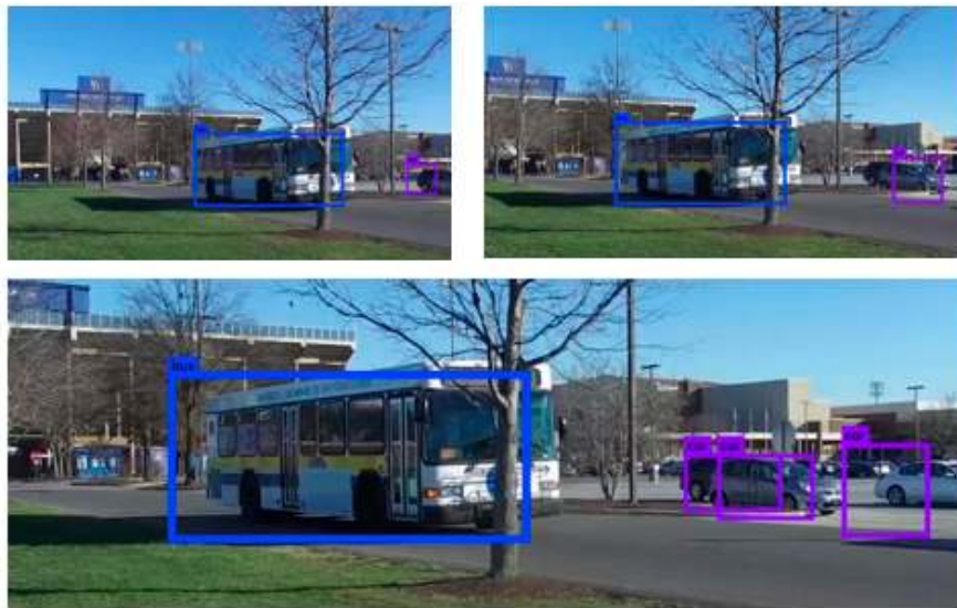
Figure 5. Sample detection of the two object classes: bus (blue bounding box) and car (blue-violet bounding box) from the video sequence obtained by drone and recognized in real time by CNN trained on aerial images.
