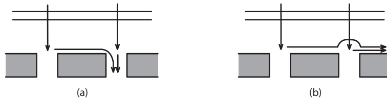
Fig. 4. Schematic view of two transmission mechanisms for a plasmon excited at one slit interacting with another slit. (a) The interference of excited surface plasmons with the incident field. (b) The interference of plasmons excited at different slits.
