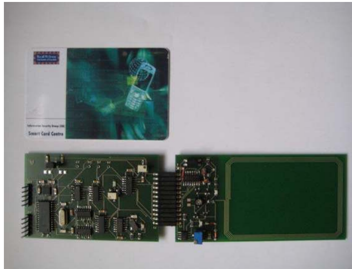
Figure 7 Custom built NFC card emulator (see online version for colours)
