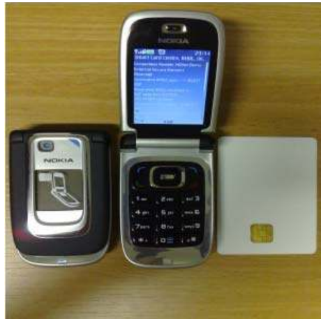
Figure 10 Cloned mobile phone token, skimmer phone and test card (dual-interfaced) (see online version for colours)
