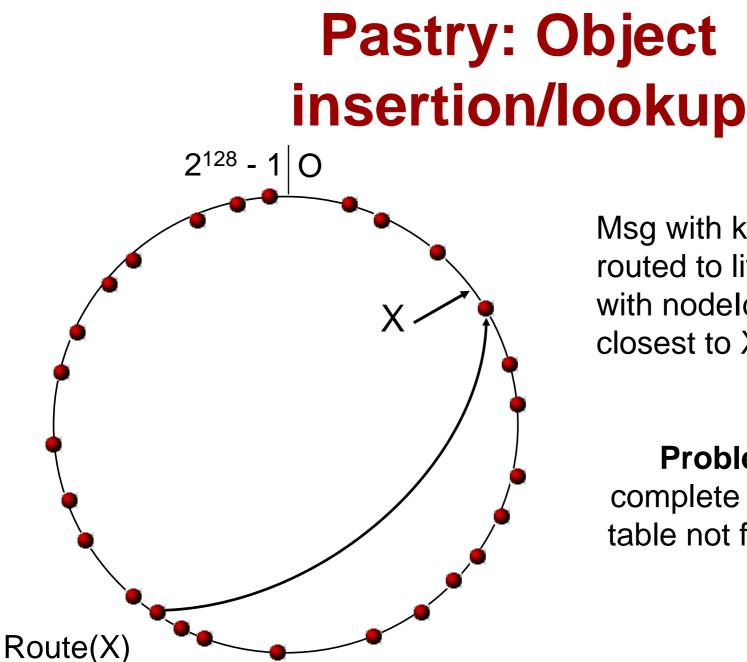
Msg with key X is routed to live node with nodeld closest to X
