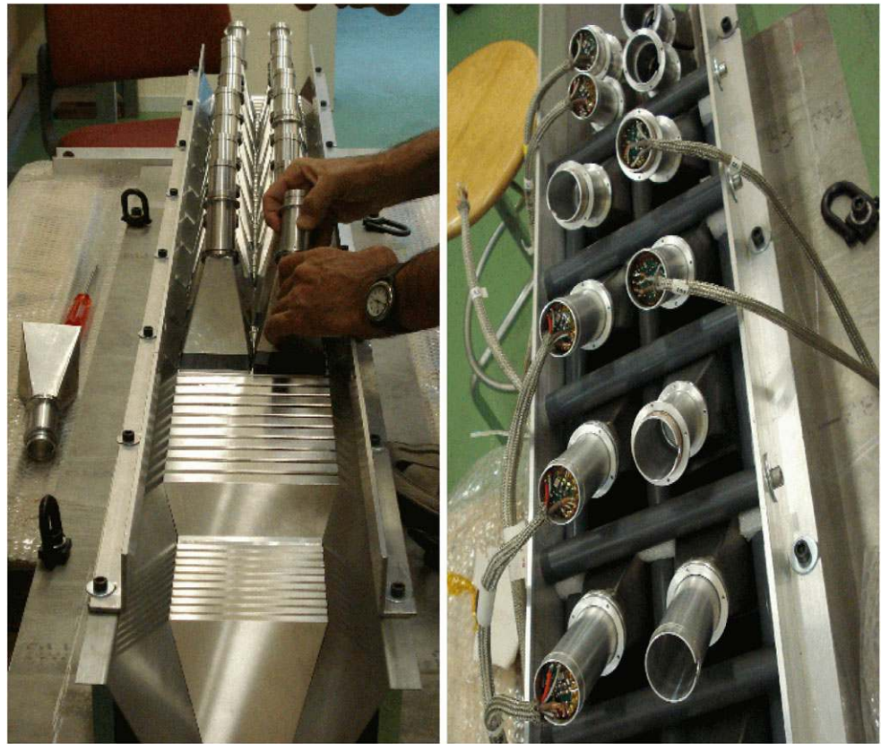
Fig. 1 CASTOR tungsten/silica quartz plates ( left ) and photomultipliers on top of the light guides ( right ) as installed on the prototype calorimeter that was beam tested in 2007 at SPS
