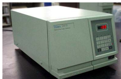
Figure 10. Refractive Index Detector
