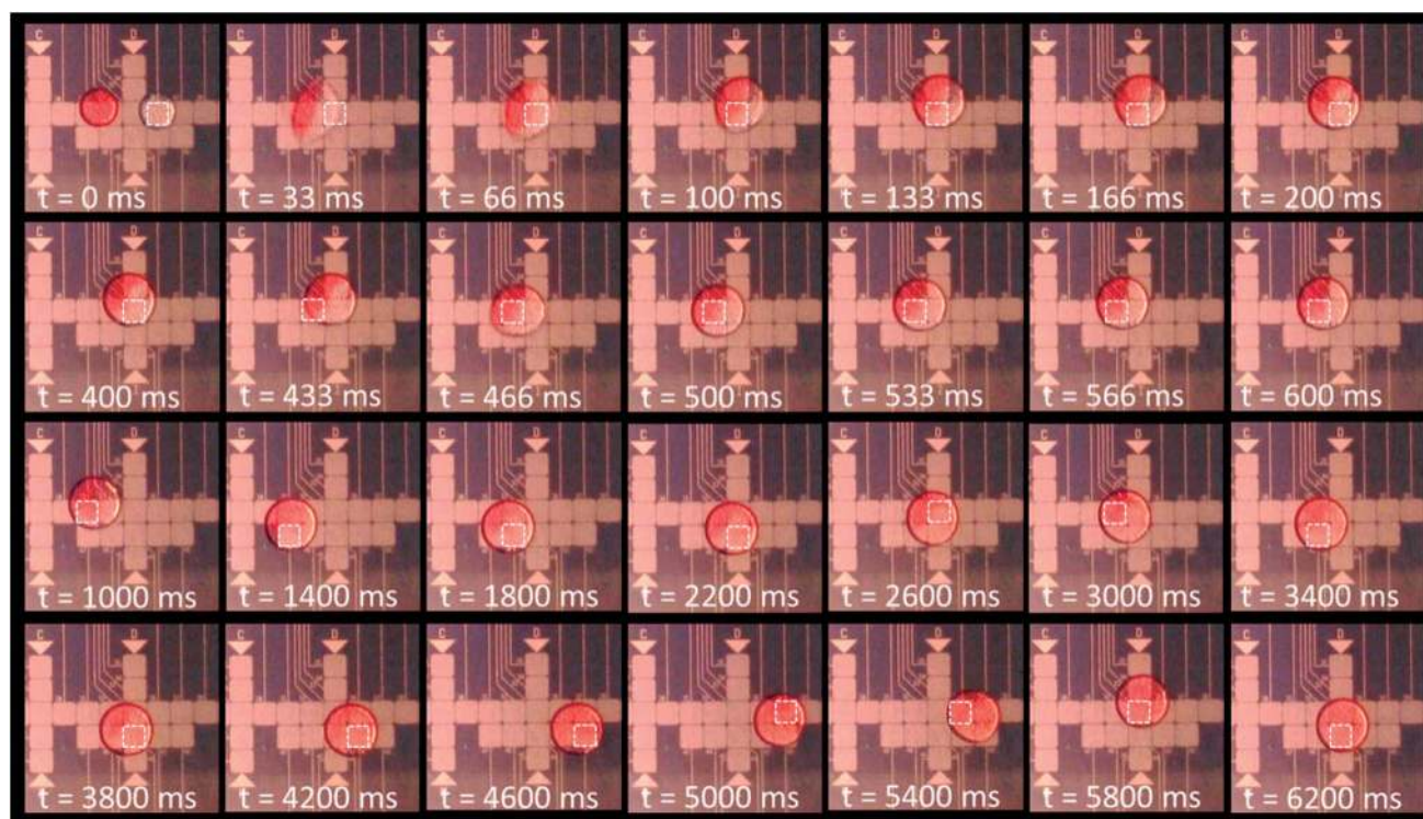
Fig. 9 Timed video frames of two 5 \mu\text{l} droplets merging and mixing in a region of a parallel-plate superhydrophobic DMF device. Both droplets are DI water solutions; the left one is pre-mixed with New Coccine dye. The white-dash contoured pads represent the energised pad. The first row shows the 30-fps frame-by-frame record of the two droplets merging together. The second row displays the frame-by-frame record of the merged droplets' actuation from one pad to one another until the complete stabilisation of the droplet. Finally, the third and fourth row (from t = 1000 \text{ ms} to t = 6200 \text{ ms} ) show the step-by-step mixing of the droplet; every frame is recorded after complete stabilisation of the droplet on the energised pad.
