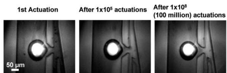
Fig. 7. PLACS reliability evaluation. A laser-induced cavitation bubble (imaged at 3 μs after laser pulse arrival) could be repeatedly produced >100 million times without showing significant bubble pattern alteration or microchannel degradation. The pulsed laser repetition rate was 10 kHz.
