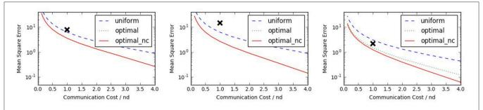
**FIGURE 1** | *Trade-off curves* between communication cost and estimation error (MSE) for four protocols. The plots correspond to vectors  $X_i$  drawn in an i.i.d. fashion from Gaussian, Laplace, and  $\chi^2$  distributions, from left to right. The black cross marks the performance of binary quantization (Example 4).
