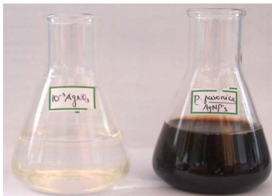
Fig. 1. Erlenmeyer flasks containing bio-synthesized silver nanoparticles by Padina pavonica , before reaction (left) after reaction (right)
