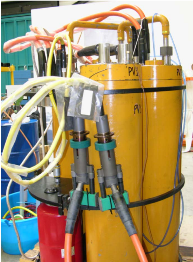
Fig. 5. Fully assembled internal vessels of the Junction Box.
