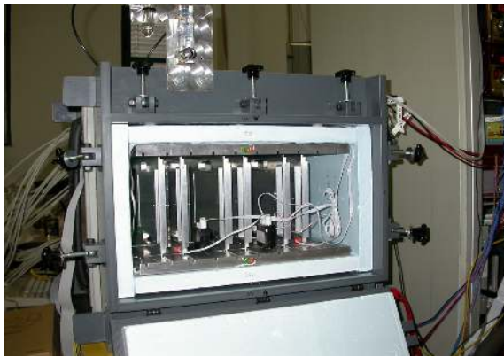
Figure 6: The Vienna cooling box filled with six modules ready for a LT test.
