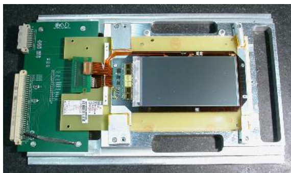
Figure 2: TIB Layer 3 module mounted on the aluminium test plate and connected to interface cards.
