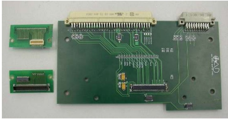
Figure 11: Erni-nais adapter (on the left of the picture, top and bottom side card views) and VUTRI adapter (on the right of the picture, top side card view).
