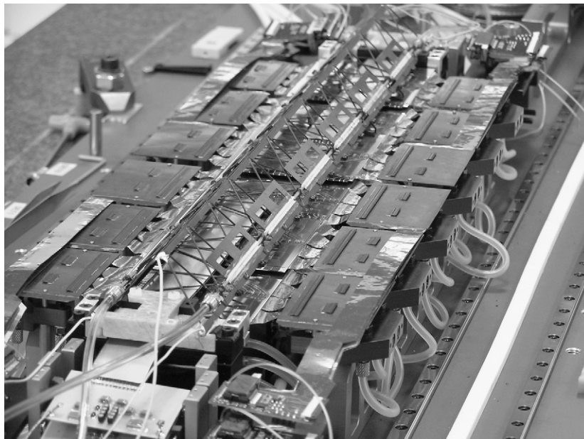
Fig. 7. The SDD ladder placed on the six aligned modules (ITS layer 3).
