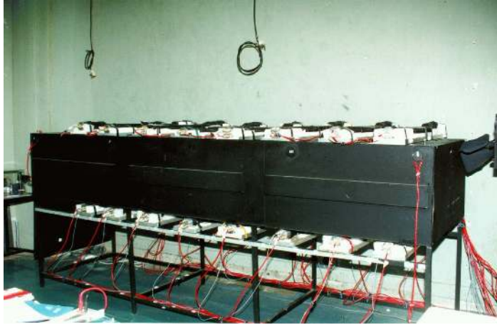
Figure 20: The setup for testing HO trays with cosmic muons.
