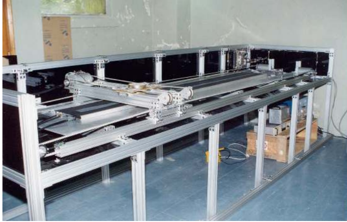
Figure 18: The setup of the radioactive XY scanner which is used to test the HO trays
