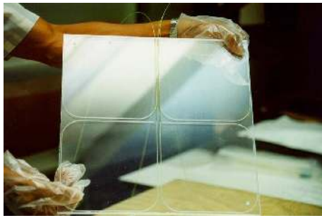
Figure 9: View of a typical tile of HO with WLS fibres inserted in the 4 \sigma -grooves of the tile
