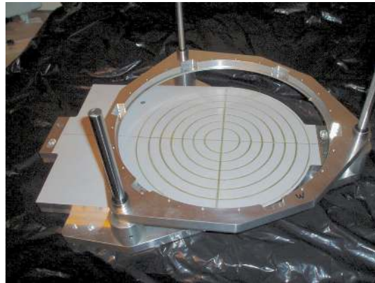
Figure 7: (a) Photograph of the vacuum chuck in position on the linear stage. The circular and diagonal grooves cut in the white Teflon sheet distribute the vacuum across the doublet layer. The photograph also shows the microscope head; and (b) Photograph of the vacuum chuck in position on the gluing jig.
