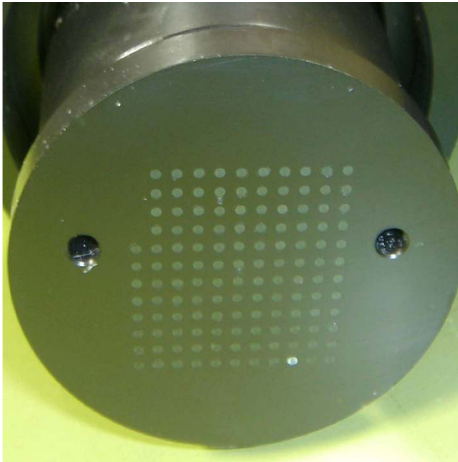
Figure 19: Photograph of the connector surface taken with strobe illumination. Reflected light is seen in a fibre at the bottom.
