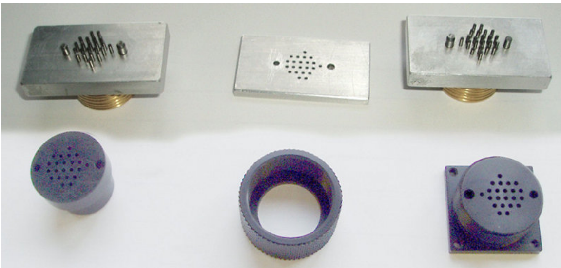
Figure 21: The station connector gauge set. The gauges are arranged in a row at the top of the photograph. The left- and right-hand gauges were used to check the connector part shown directly below. The ‘gauge gauge’ shown in the centre of the top row is used to ensure that the pins in the two gauges are precisely matched.
