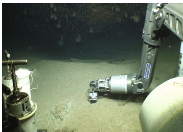
Figure 2. Sediment push core samples collected with the Global Explorer remotely operated vehicle (GEX-ROV). The GEX-ROV manipulator arm and core tube are in foreground. The Anona shipwreck's stern is in the background. Cores were collected within 2 m of each shipwreck and at distances of 75–200 m away, depending on the site. Photograph taken by the GEX-ROV, operated by Deep Sea Systems International during expedition PE14–15, and provided by the Bureau of Ocean Energy Management.
