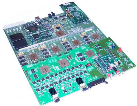
Figure 4: the L0DU mezzanine plugged on a TELL1 board
